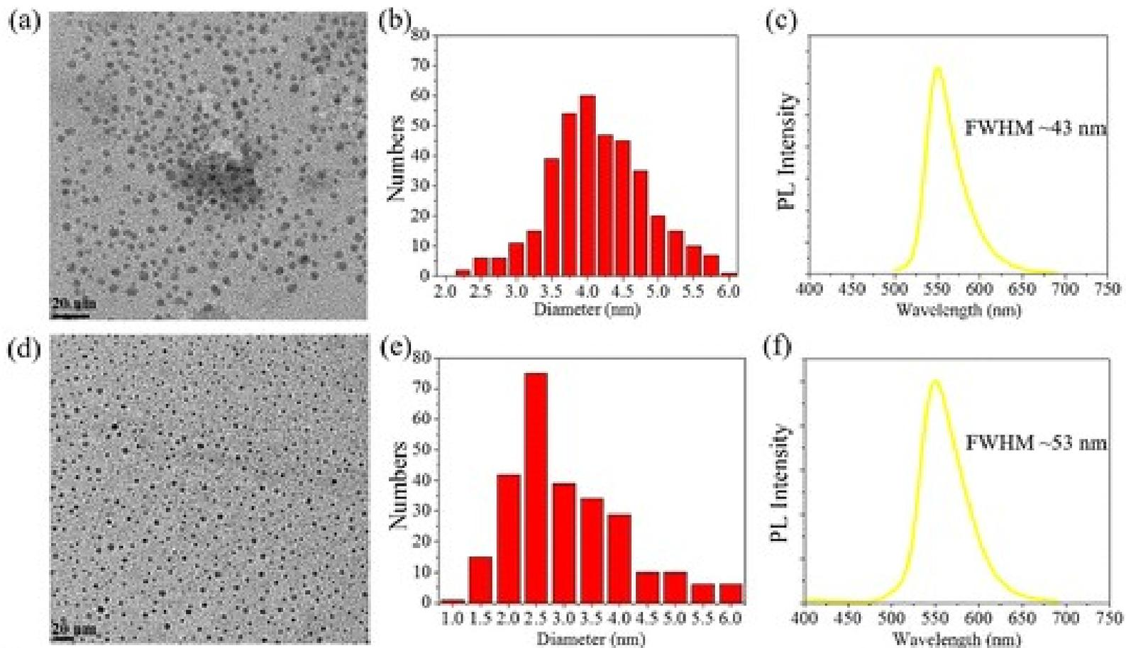
Figure 3. Si NPs of different sizes and their size-independent PL. (a and b) TEM graph and size distribution of Si NPs with average diameter of 4.1 nm. (c) PL spectrum of the 4.1 nm Si NPs. (d and e) TEM graph and size distribution of Si NPs with average diameter of 2.8 nm. (f) PL spectrum of the 2.8 nm Si NPs (scale bar in TEM images: 20 nm).
