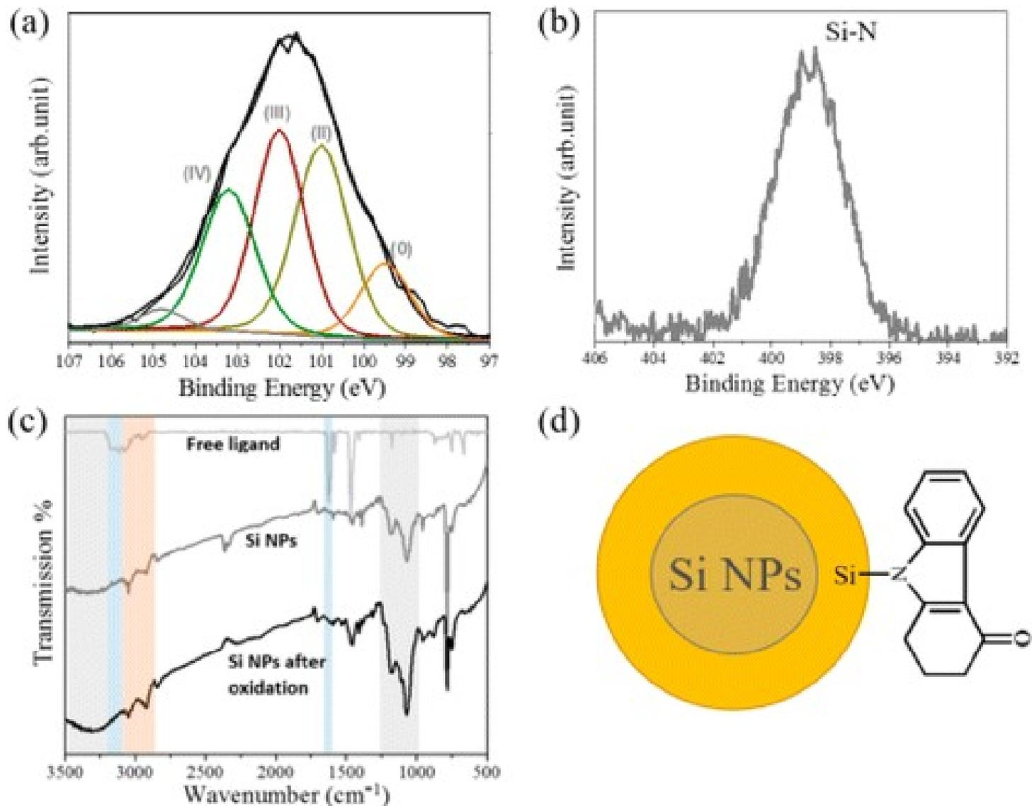
Figure 2. Characterization of the On-Si NPs. X-ray photoemission spectra of (a) Si 2p region and (b) N 1s region. (c) FTIR spectra of the On-Si NPs and On-ligands. (d) Structure model of the On-Si NPs.
