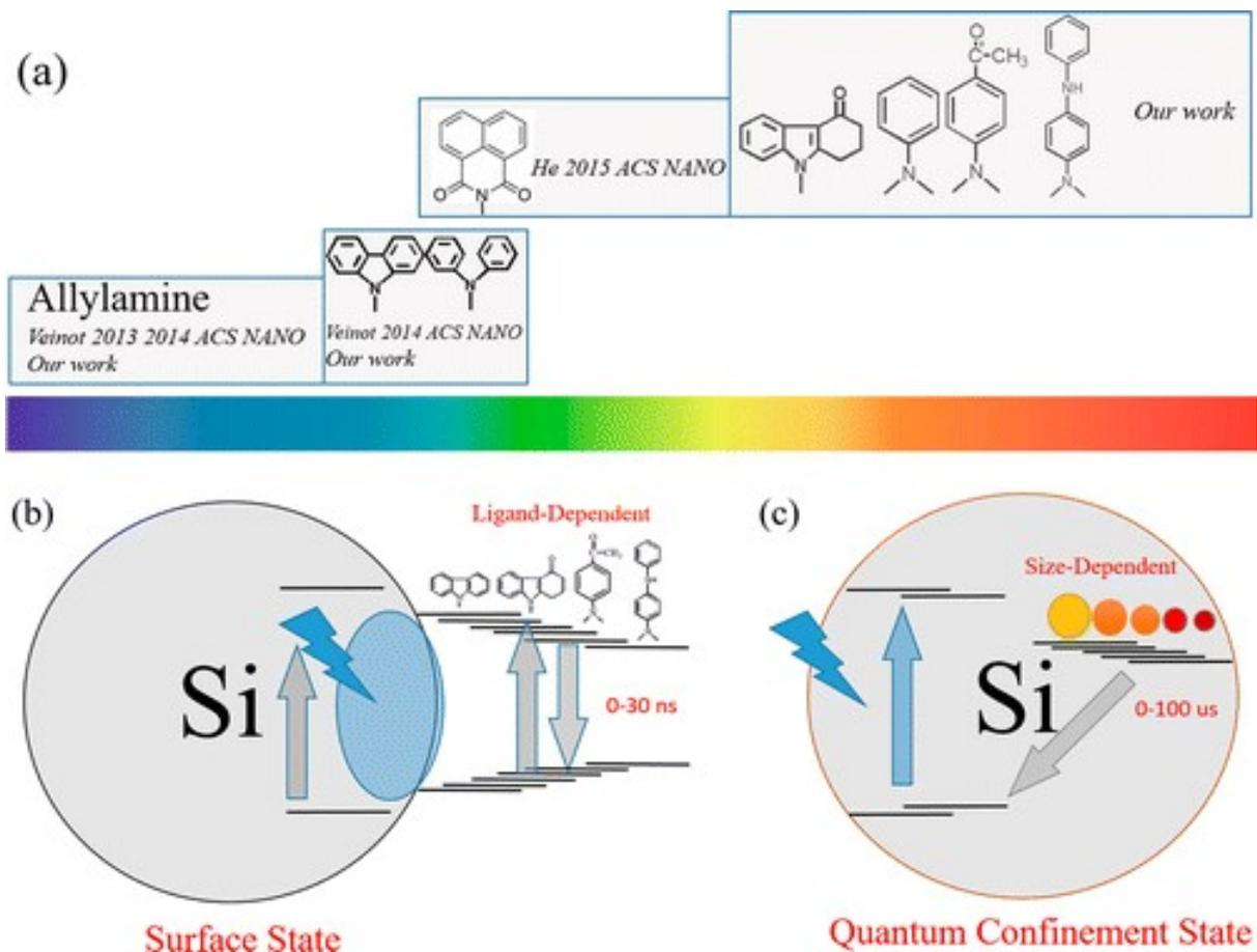
Figure 7. PL mechanism of surface nitrogen-capped Si NPs. (a) Spectral tunability of surface nitrogen-capped Si NPs from different fabrication methods that follow the ligand structure law. (b) Scheme of the surface PL from surface nitrogen-capped Si NPs. (c) Scheme of the quantum confinement PL from conventional Si quantum dots, as a contrast.
