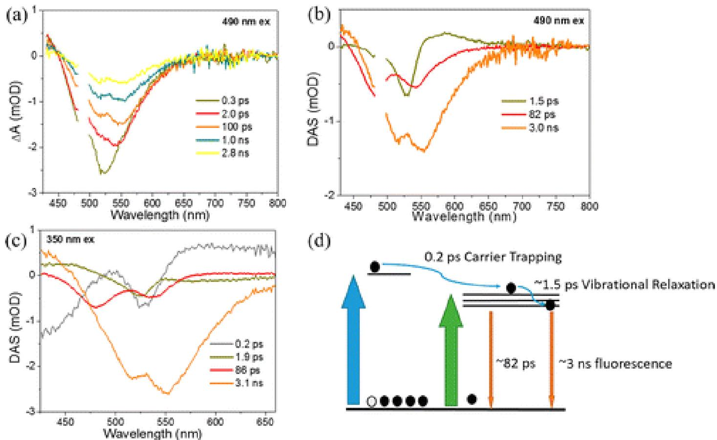
Figure 4. Femtosecond transient absorption study of the On-Si NPs. (a) Time evolution of transient absorption spectra (excitation at 490 nm). (b) Decay-associated spectra (DAS) obtained from the global analysis (excitation at 490 nm). (c) DAS obtained from the global analysis (excitation at 350 nm). (d) Energy diagram of the On-Si NPs.
