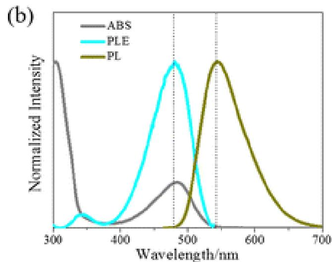
Figure 6. Influence of ligand amount on the optical properties of Si NPs. (a) Calculated electron density distribution of the HOMO and LUMO of the Si NPs with different amounts of On-ligand. (b) PL, PLE, and absorption spectra of the green-yellow-emitting On-Si NPs obtained by reducing the amount of added surface ligand during reaction.
