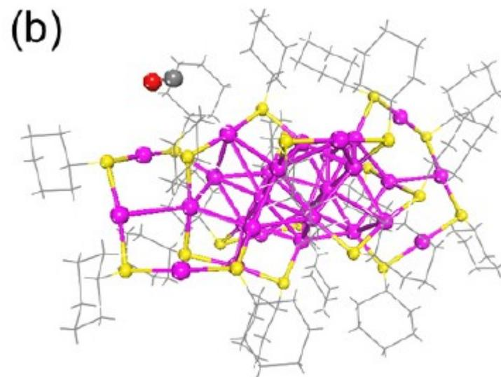
**Figure S4.** Most stable adsorption geometry of CO on (a) Au<sub>28</sub>(SPh-<sup>t</sup>Bu)<sub>20</sub> and (b) Au<sub>28</sub>(S-*c*-C<sub>6</sub>H<sub>11</sub>)<sub>20</sub>. Au, pink; S, yellow; C, grey; O, red; R groups, lines.
