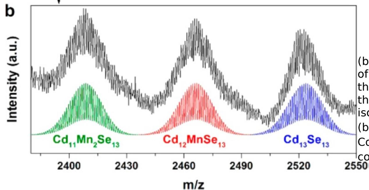
(b) High-resolution mass spectrum of the main peaks indicated with the dashed box in panel a. Below the measured data, calculated isotopic distributions of  $\text{Cd}_{13}\text{Se}_{13}$  (blue),  $\text{Cd}_{12}\text{MnSe}_{13}$  (red), and  $\text{Cd}_{11}\text{Mn}_2\text{Se}_{13}$  (green) are shown for comparison.
