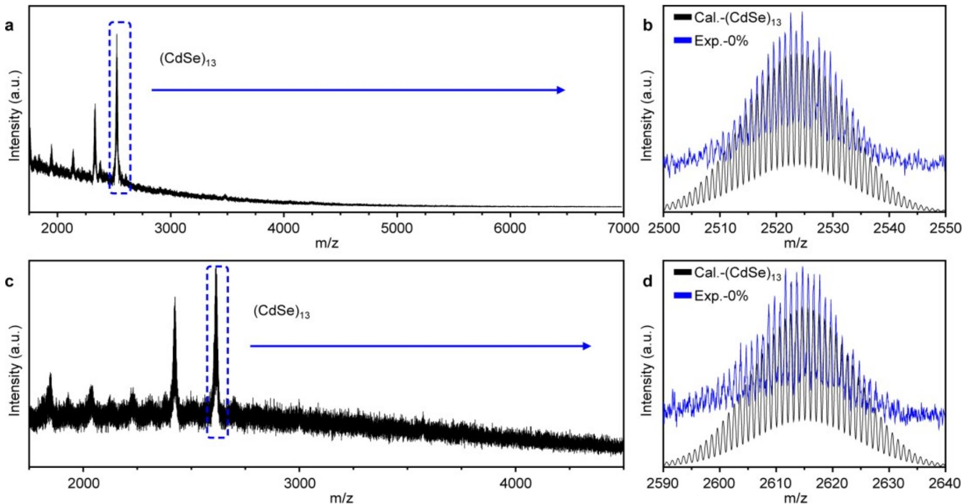
a) LDI-TOF MS spectrum of undoped  $(\text{CdSe})_{13}$  clusters ionized by chlorine anions. (b) The expansion around the main peak in panel a (blue rectangle) in isotopic resolution. (c) LDI-TOF MS spectrum of undoped  $(\text{CdSe})_{13}$  clusters ionized by iodine anions. (d) The expansion around the main peak in panel c (blue rectangle) in isotopic resolution.
