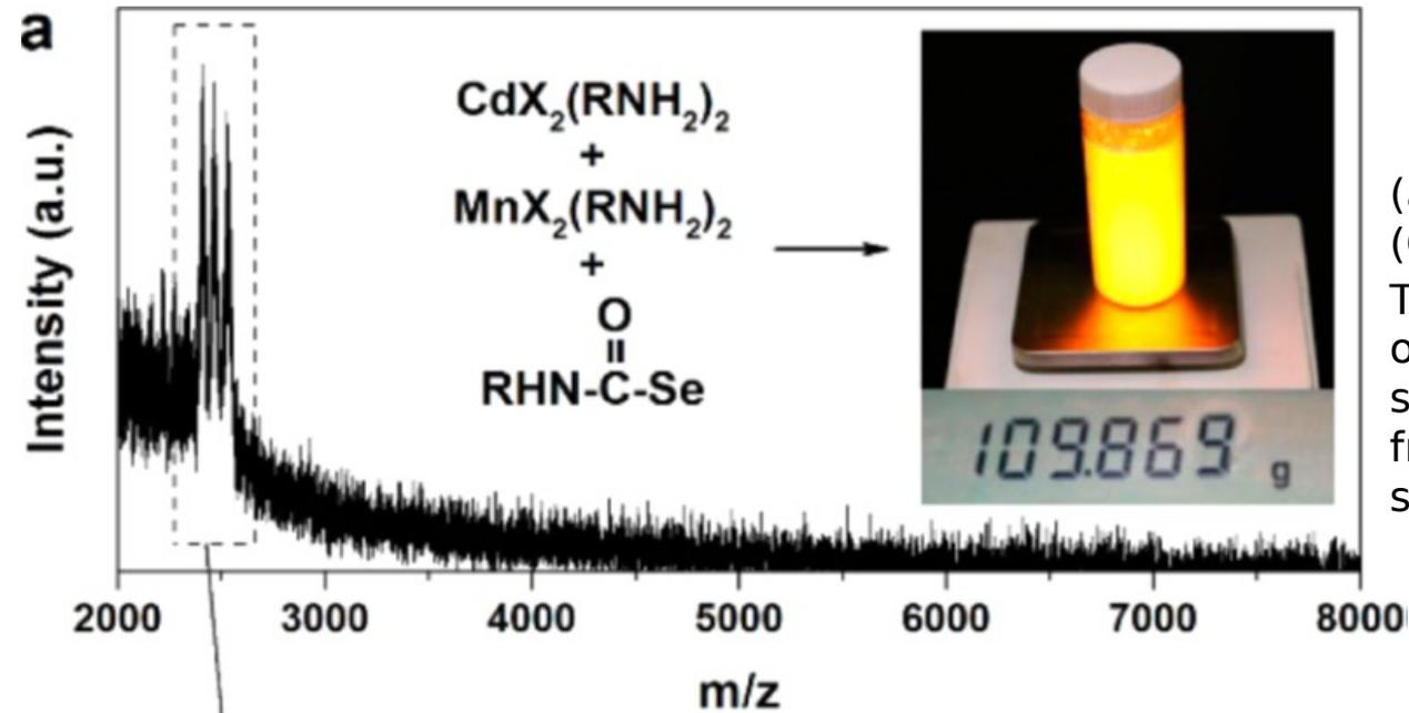
(a) Mass spectrum of  $\text{Mn}^{2+}$ -doped  $(\text{CdSe})_{13}$  clusters ionized with  $\text{Cl}^-$ . The average doping concentration of the clusters is 7%. The inset shows the amount of the product from a single batch large-scale synthesis.
