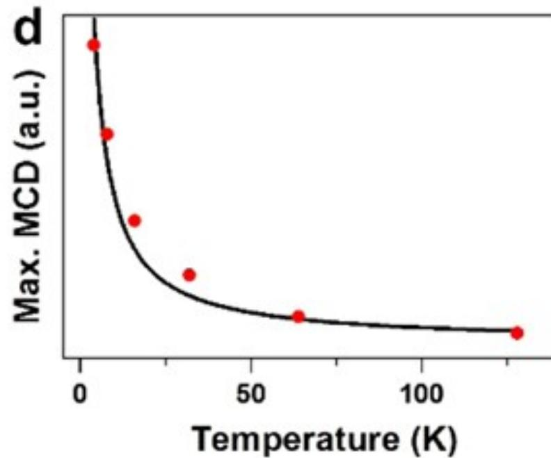
(c) Temperature-dependent MCD spectra of 4% Mn<sup>2+</sup>-doped clusters under the magnetic field of 1.6 T. (d) Maximum amplitude of the MCD signal in panel c as a function of temperature. The black curve represents a theoretical Brillouin fit.
