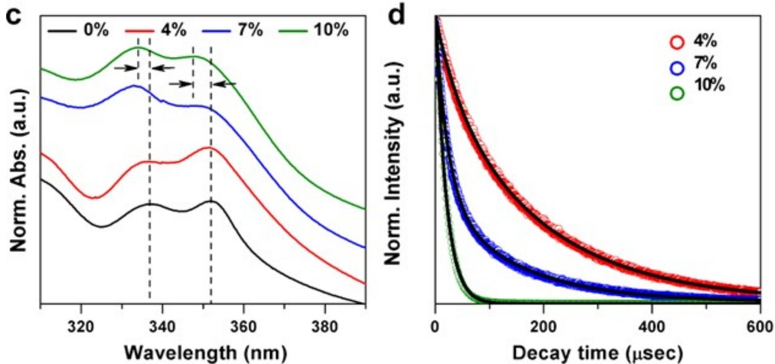
(c) Absorption spectra of  $(\text{CdSe})_{13}$  clusters with various doping concentrations. The arrows indicate the shift of the absorption peak positions. (d) Time-resolved luminescence decay at 600 nm from  $\text{Mn}^{2+}$ - $(\text{CdSe})_{13}$  clusters with different doping concentrations. Decay data are overlapped with the corresponding fitting curve (black).
