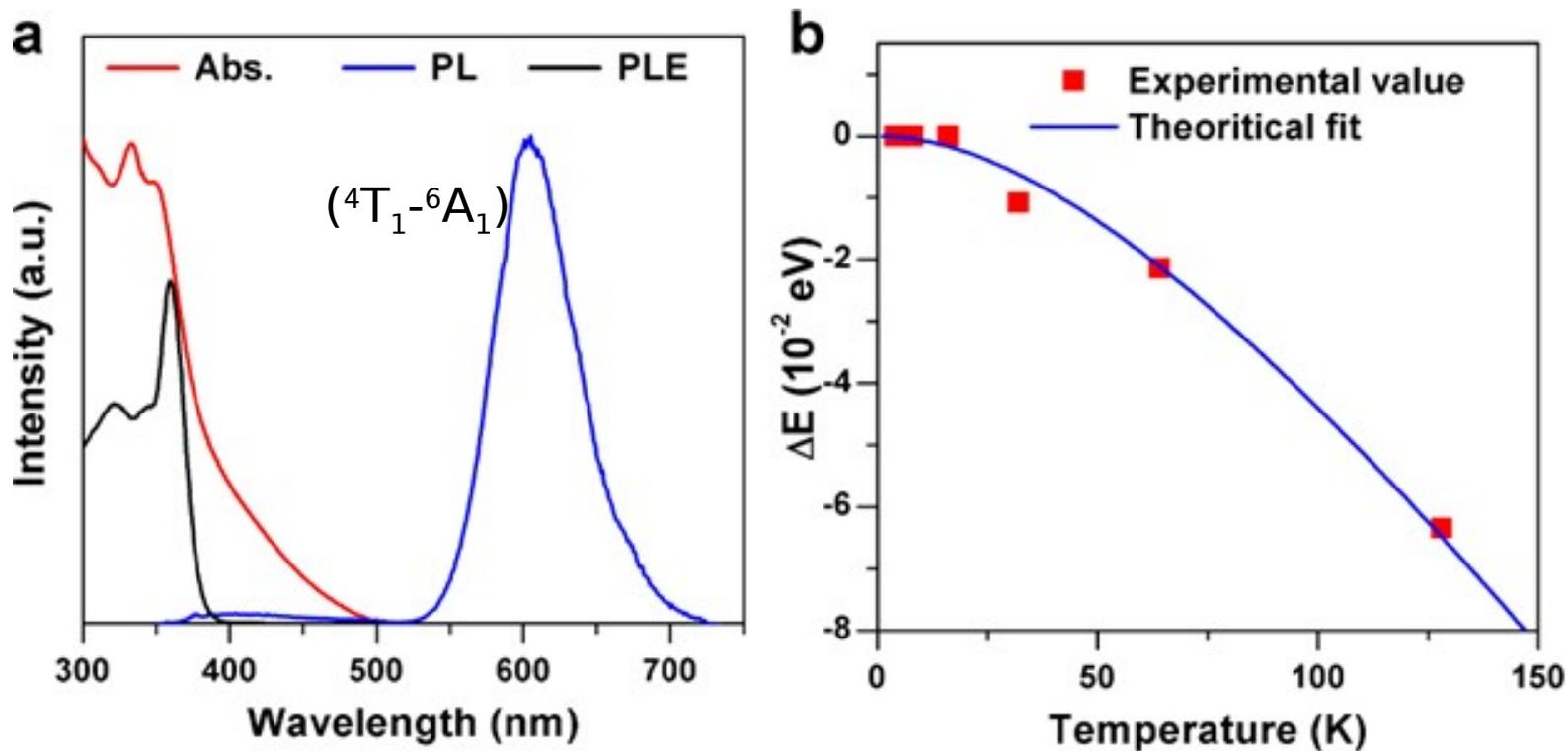
Optical properties of  $Mn^{2+}$ -doped  $(CdSe)_{13}$  clusters. (a) Spectra of absorption, PL, and PLE (detected at 600 nm) from as-synthesized (n-octylamine capped) 7%  $Mn^{2+}$ -doped  $(CdSe)_{13}$  clusters. (b) Energy shift of the absorption edge of  $Mn^{2+}$ -doped  $(CdSe)_{13}$  clusters as a function of temperature. The theoretical fitting curve is calculated by using the Varshni law with the parameters  $\alpha = 11 \times 10^{-4}$  eV  $K^{-1}$  and  $\beta = 150$  K.
