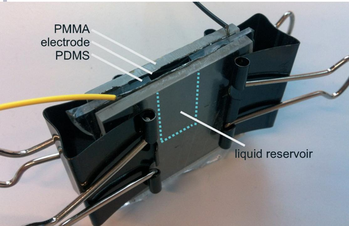
Photo of the macrofluidic cell (a) and schematic cross-section of the cell as seen from the top (b). The cell consists of two polymethyl methacrylate (PMMA) sheets separated by a u-shaped spacer of thickness 2.25 mm. The liquid volume of the liquid reservoir formed by the spacer is 0.45 ml.
