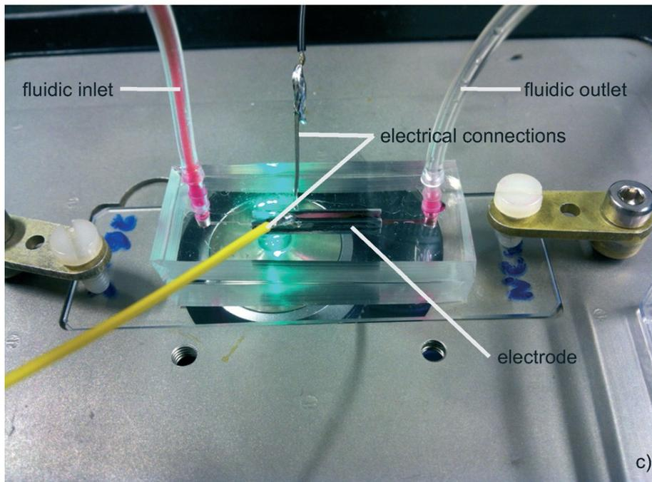
The distance between the electrodes **-1.5 mm**.
