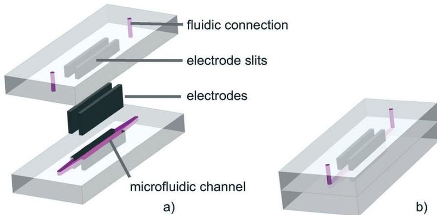
a) Exploded view of the chip. The fluidic channels are colored in violet. The carbon electrodes are colored black.
