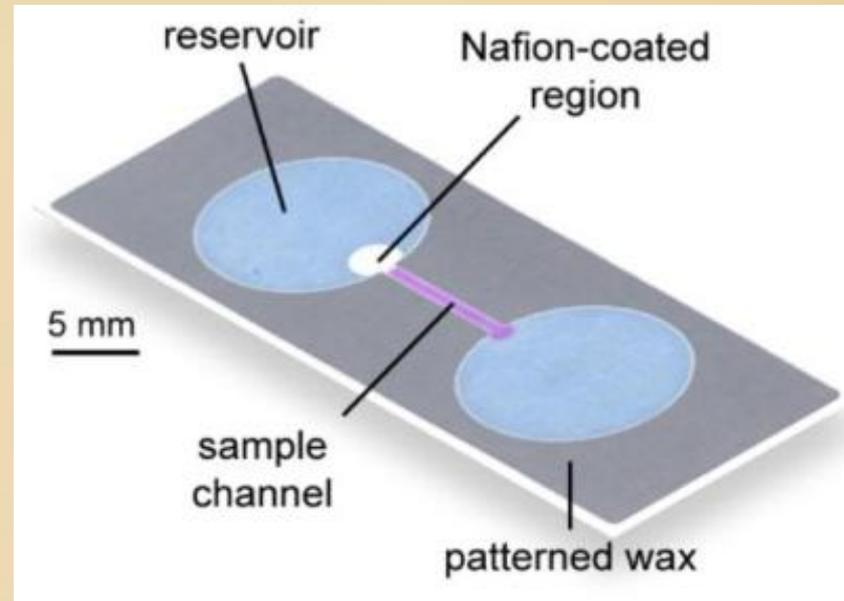
*Device schematic with reservoirs (blue), sample channel (purple), and Nafion-coated region (white)*
