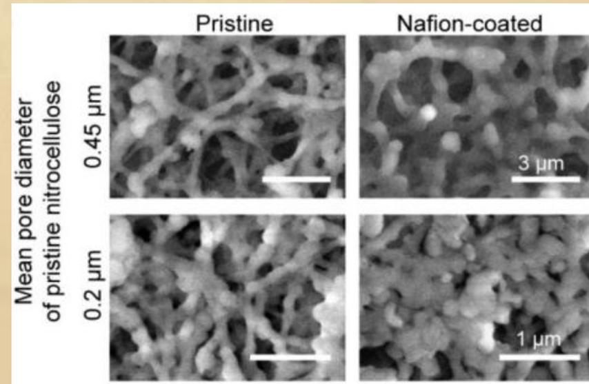
*Environmental scanning electron microscopy images of nitrocellulose paper with and without Nafion coating*
