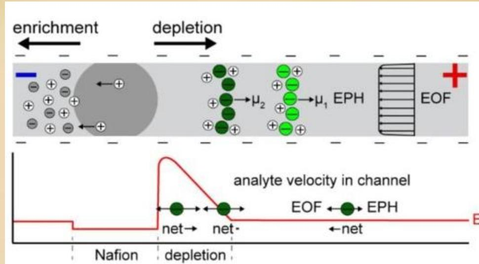
*Schematic of ICP enrichment and depletion effects under applied voltage. Net movement of analytes is governed by electrophoretic migration (EPH) and electroosmotic flow (EOF), in response to the local electric field strength,  $E$ .*
