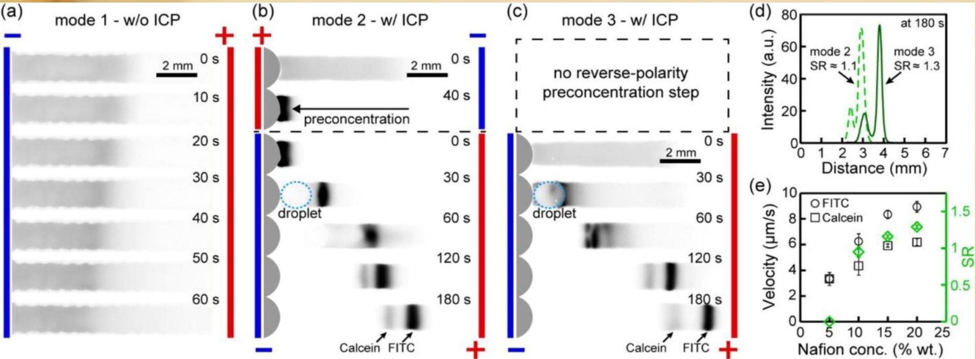
(a) Operating mode 1—transport without ICP. (b) Operating mode 2—preconcentration and separation with switching-polarity ICP. (c) Operating mode 3—direct preconcentration and separation with ICP. (d) Separation resolution (SR) in modes 2 and 3. (e) Effect of Nafion concentration (% wt.) on the separation process. Data points are the average of  $n = 3$  measurements with error bars as one standard deviation. Images have been contrast adjusted for presentation (similarly in each case).
