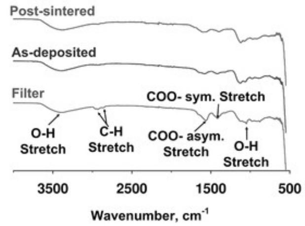
Schematics of a) a photodetector substrate and b,c) flame spray pyrolysis synthesis and aerosol self-assembly of d) ultraporous films made of electron-depleted ZnO nanoparticles at 20 cm height above the burner. e) The XRD patterns and FTIR spectra of the ZnO particles collected on the filters and substrate before and after sintering.
