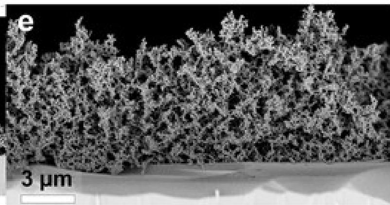
Optical transmittance spectra of ultraporous ZnO films, Inset: Optical images of ZnO films deposited for 15 and 100 s on glass substrates placed over a printed paper. SEM images of an exemplary film deposited for 100 s on a glass substrate reveal a highly porous and uniform (b,c) top surface and (d,e) cross-section.
