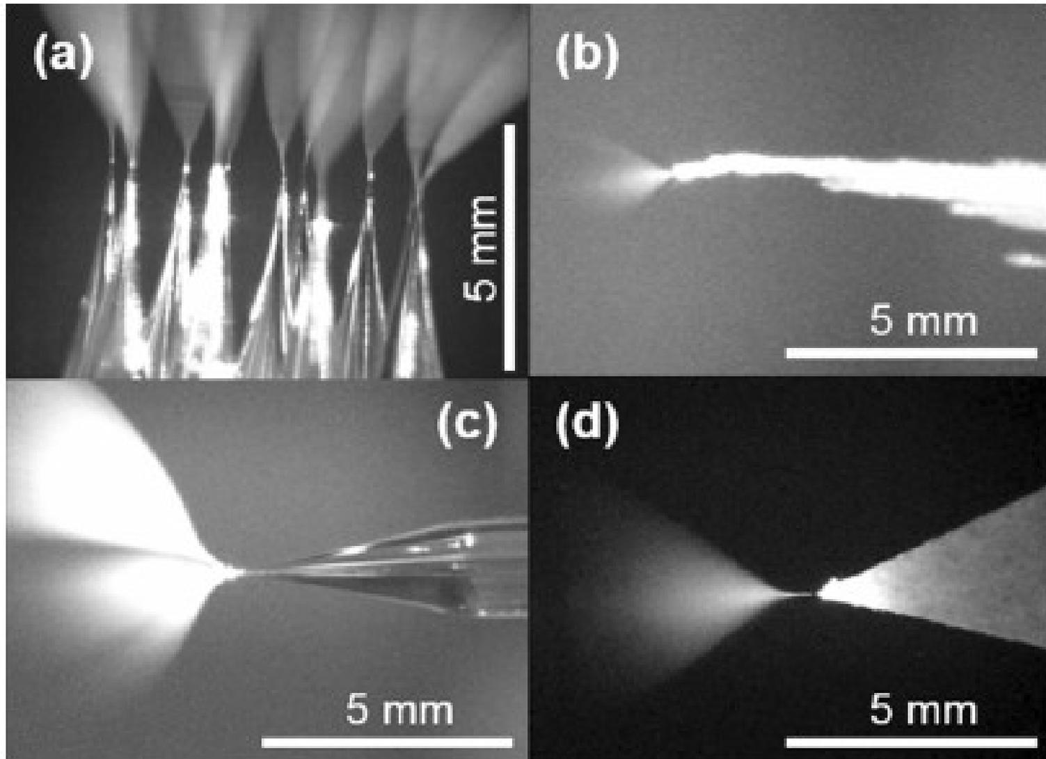
***Relay spray from several different emitters: a) bundle array of 11 nanoESI emitters; b) sharp end of a wooden pick; c) pulled thetashaped tip, and d) filter paper triangle.***
