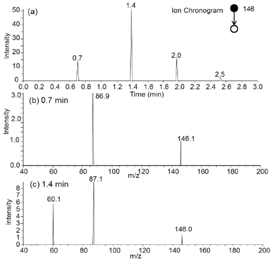
**Total instrument count (a) and MS/MS spectra (b) and (c) obtained from rESI of ~1 pL of a 0.5 ppb acetylcholine solution (estimated as 0.5 attogram, 3 zmol, 2,000 molecules) loaded into a capillary and analyzed by rESI. Four separate experiments were done as shown in the total ion count showing the repeatability and deviations in the data.**
