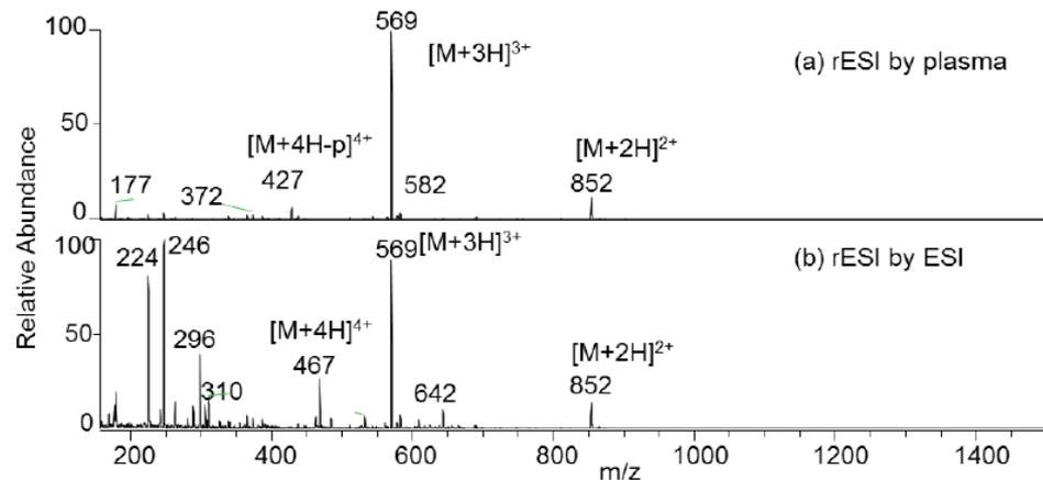
**When using a piezoelectric plasma discharge as a primary ion source in a relay experiment run in with an open secondary capillary (a), a small degree of dephosphorylation was observed for the highly charged phosphopeptide ion  $[M+4H-p]^4+$  as compared to the native forms observed by ESI or conventional nanoESI. The absolute intensity (normalized level) for (a) and (b) were  $1.1 \times 10^3$  and  $1.5 \times 10^3$  respectively.**
