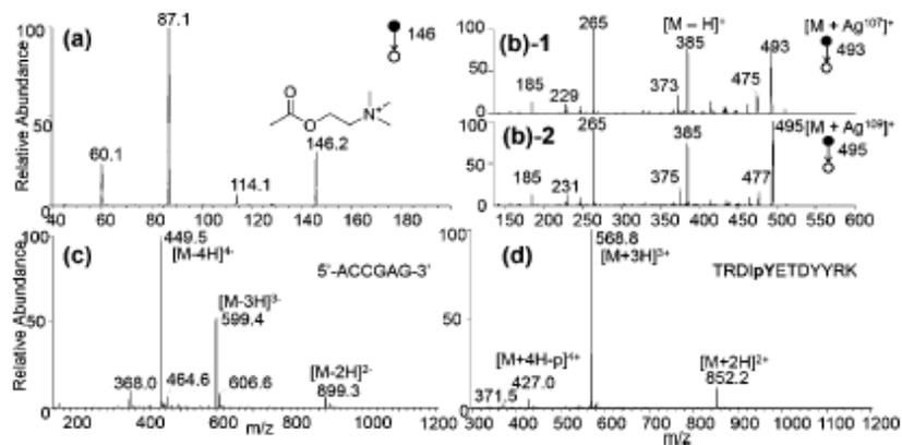
**Relay electrospray MS analysis of a) ca. 1 pL of 0.5 ppb acetylcholine, MS/MS of m/z 146. b) 100 ppb cholesterol, MS/MS of isotopic  $[M+Ag]^+$  ions, c) 1  $\mu$ M DNA oligomer in negative ion mode, and d) 1  $\mu$ M phosphopeptide.**
