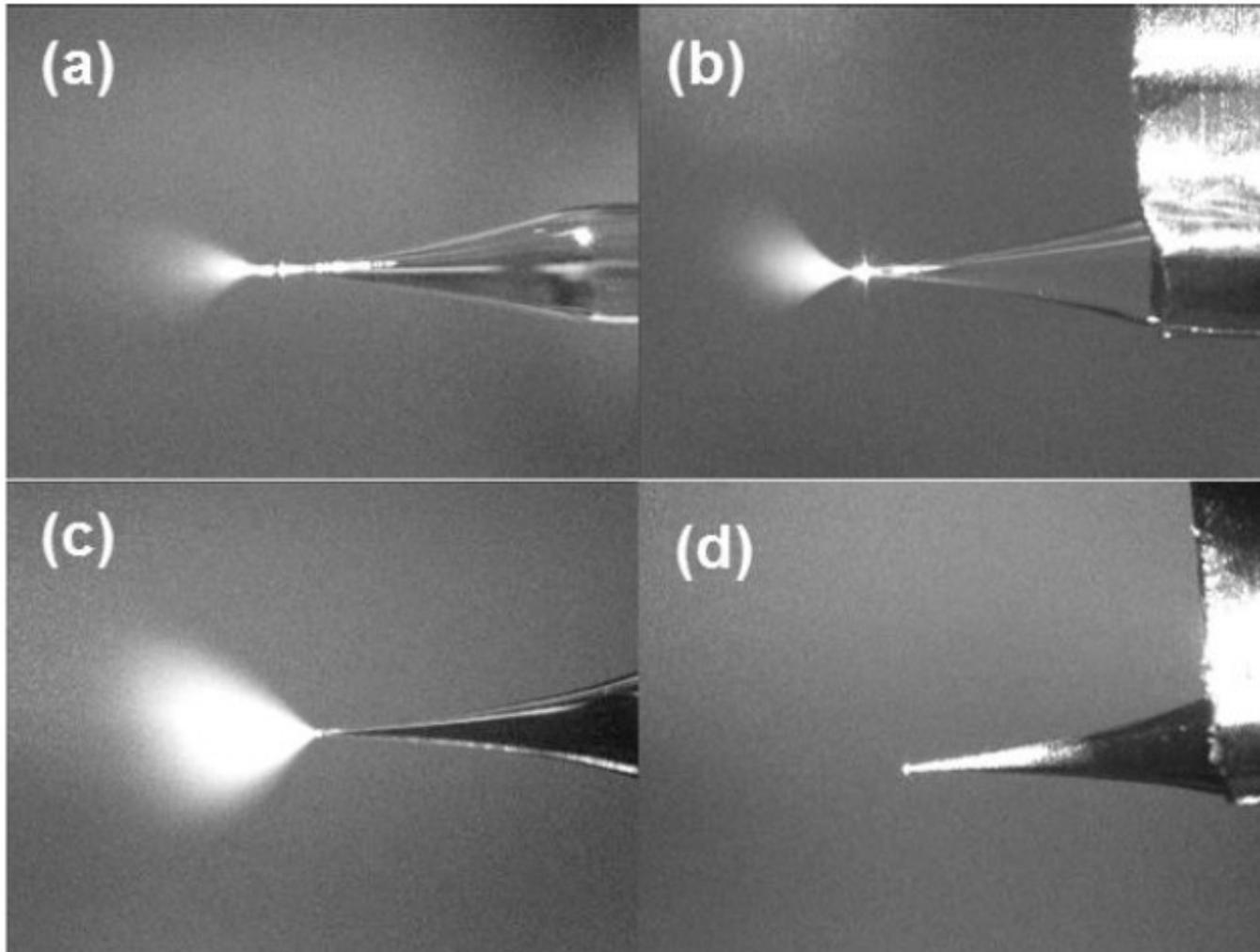
***Relay electrosprays could be generated from the distal end (a) of capillaries sealed at the proximal end; even when (b) the sealed capillary's outer wall was partially grounded using a copper tape, and (c) the capillary's outer wall was sputter coated with ~5 nm Au/Pd. Only (d) when this coated outer wall was grounded could the relay spray be avoided.***
