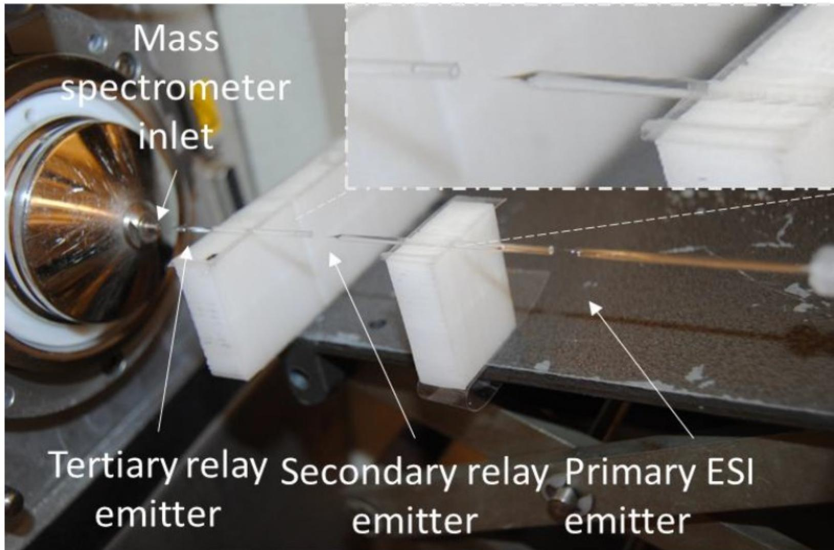
***Triple serial electrospray relay of as a demonstration of multiple stage capability. This configuration has an overall current transmission efficiency of 36%. Similarly, quadruple serial relays were constructed using a needle plasma discharge as primary ion source, with overall current transmission efficiency of only 4%.***
