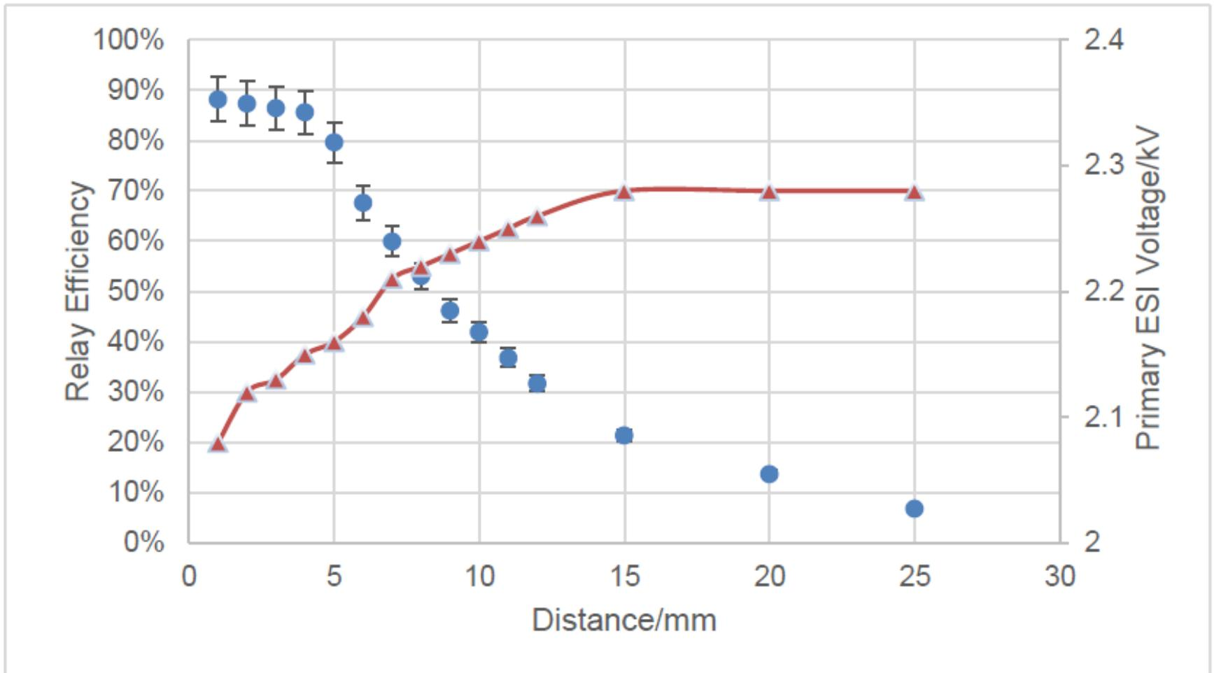
***ESI-ESI relay efficiency and primary voltage vs. emitter to emitter distance, the primary ESI current was held at 12 nA by adjusting the applied voltage (triangles), the current from the secondary (relay) ESI is presented as a percentage of the primary current (dots) for different distances (primary tip end to secondary proximal end) between the two emitters.***
