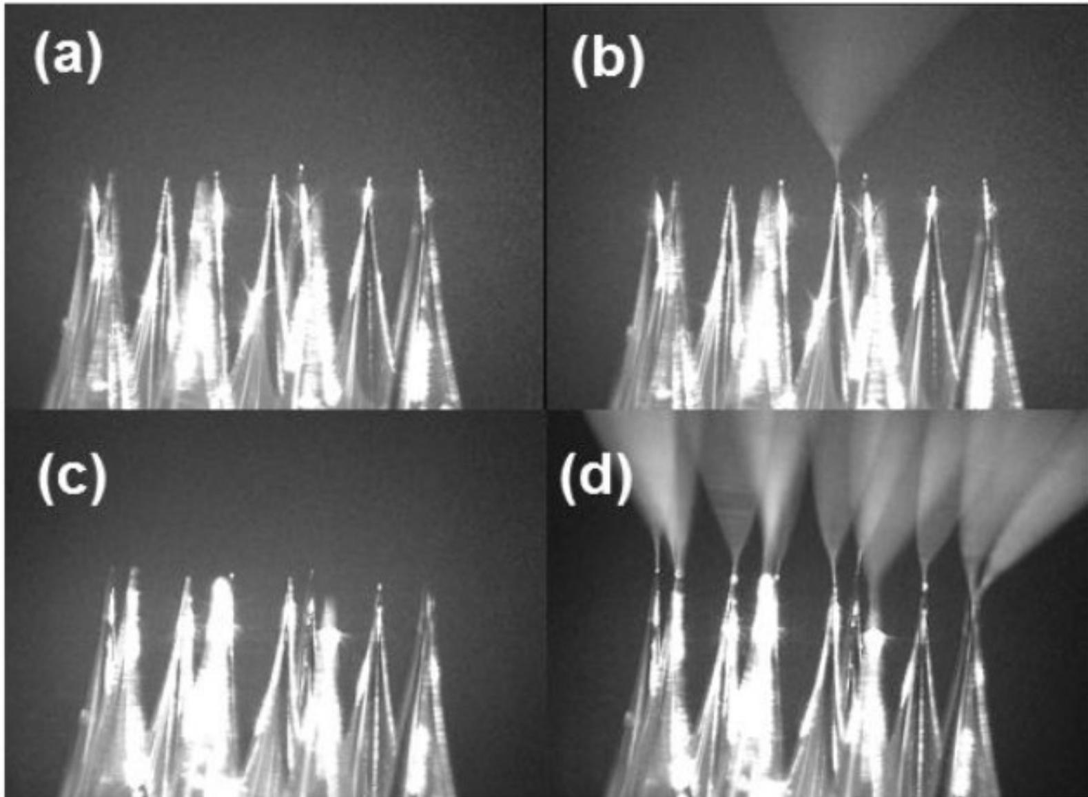
*Array of emitters (a) before and (b) upon selective triggering of one channel; (c) before and (d) upon simultaneous triggering of all 11 emitters in the array.*
