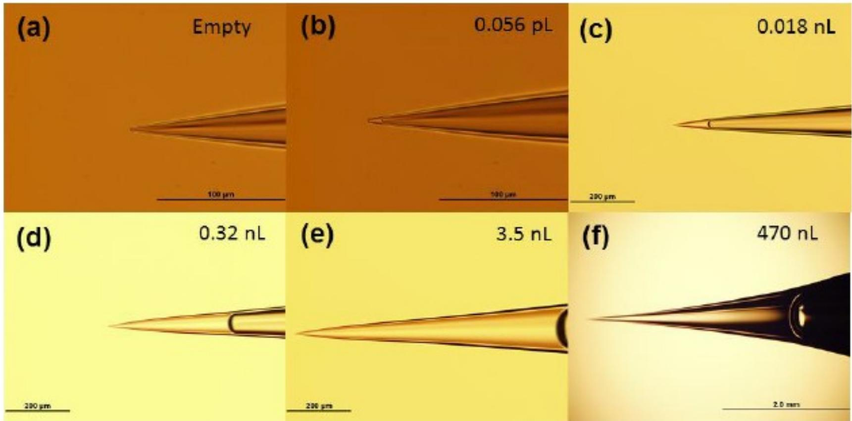
*Ultra-low volume (from sub picoliters to microliters) sample solution (to the left of the meniscus) was loaded into the sharp tip of the relay capillary. Relay electrospray phenomenon was observed for all of these loaded tips.*
