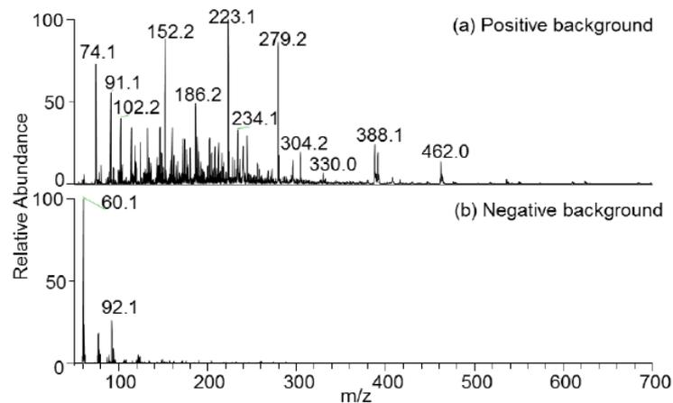
**Background ions generated by the piezoelectric discharge plasma in positive (a) and negative (b) modes in a lab environment. The discharge plasma was placed 30 cm away from the mass spectrometer inlet. The absolute intensity (normalized level) for (a) and (b) were  $1.1 \times 10^4$  and  $5.2 \times 10^4$  respectively.**
