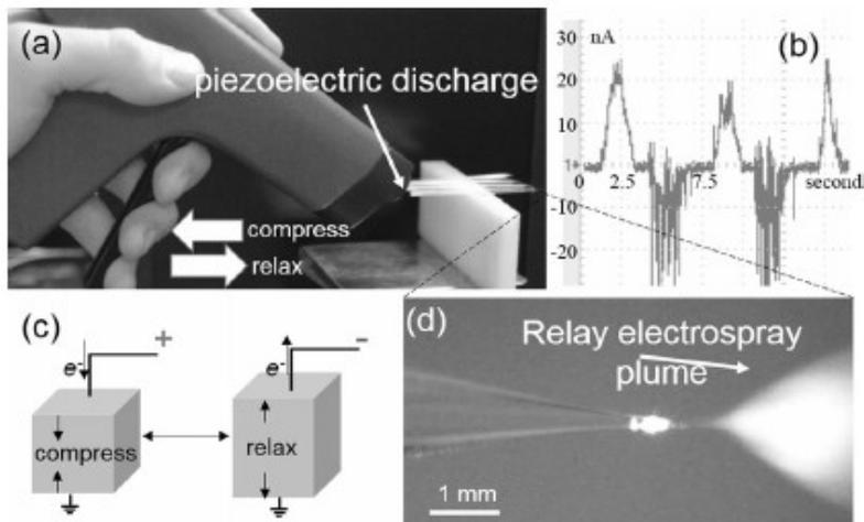
**Hand-held piezoelectric direct discharge plasma generator as primary ion source in relay ESI. a) Photograph of set-up; b) rESI current through three positive and two negative cycles; c) electrical operating schematic and d) photograph of relay spray plume.**
