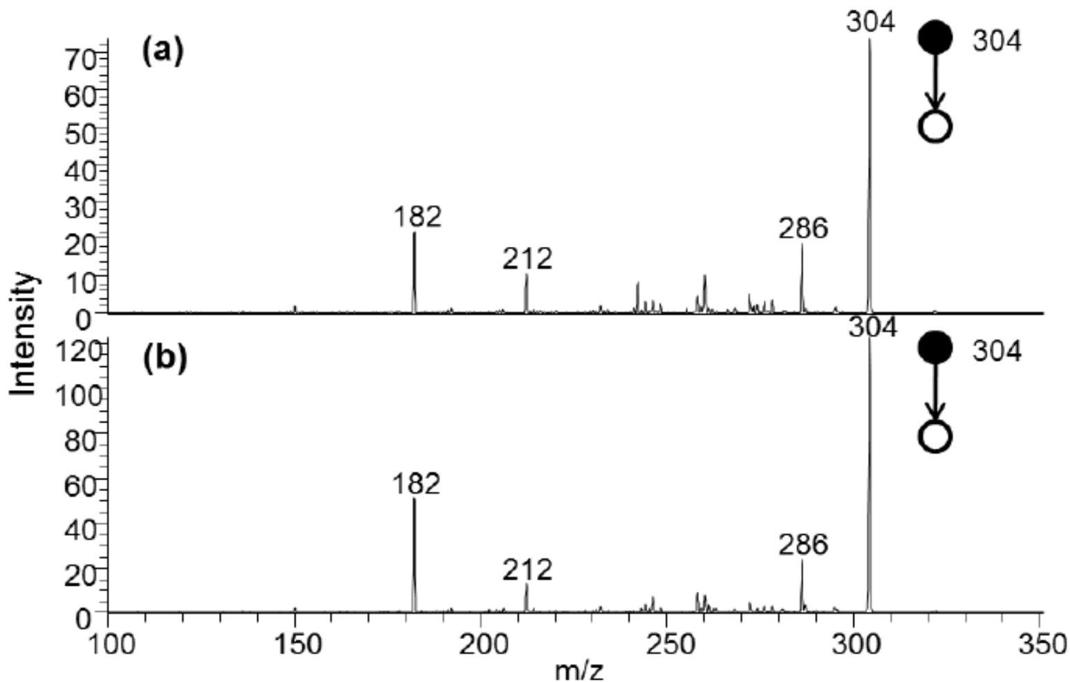
***MRM intensity (absolute intensity on y axis) from the same (1 ppb) cocaine solution from the same secondary emitter (a) after and (b) before sealing the proximal end. Comparison of the data indicates a 40% decrease in signal after sealing the end.***
