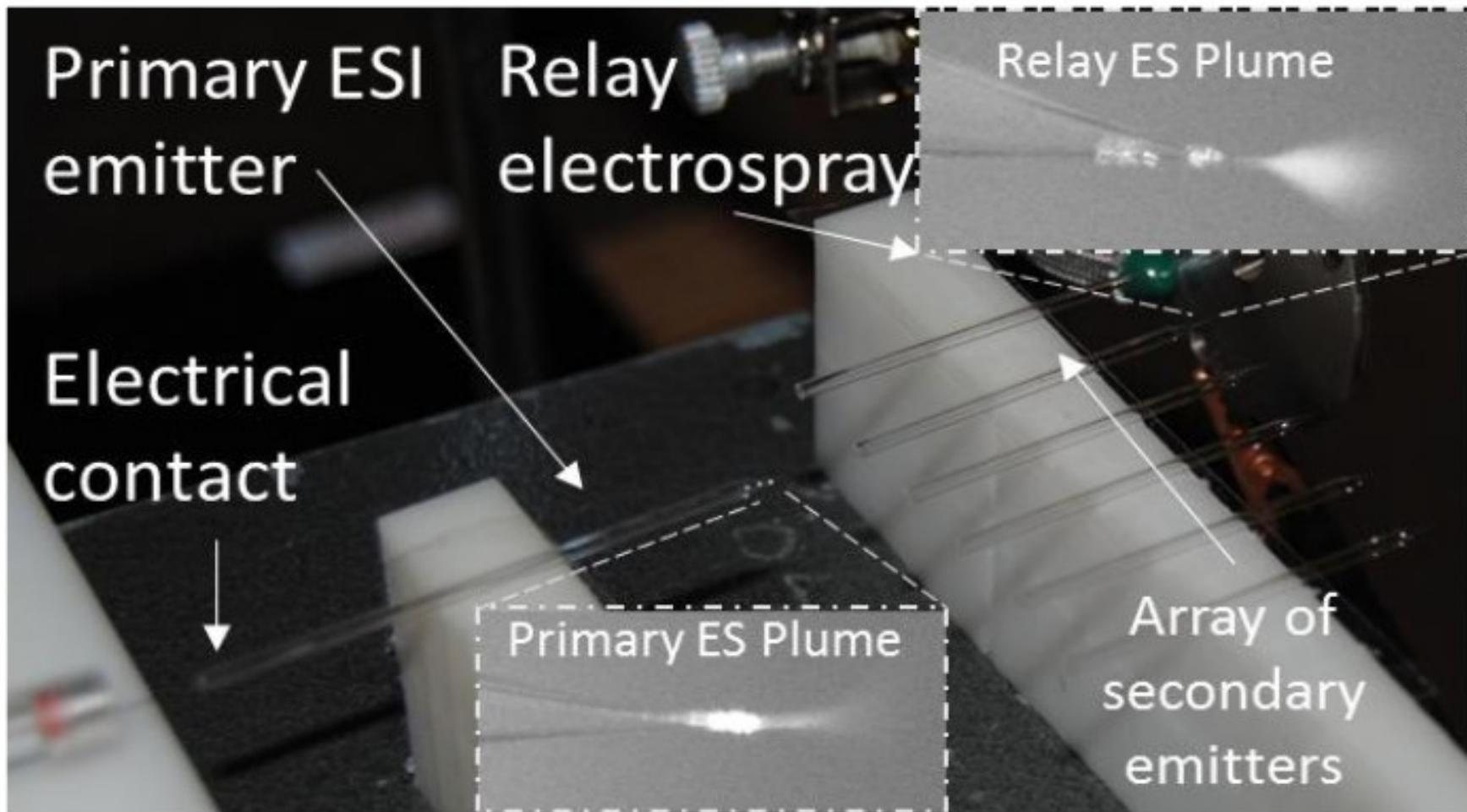
*Using a regular wire-in nanoelectrospray emitter as the primary ion source, a spray plume from the sample loading relay (secondary) tip was captured by camera under illumination. In a typical experiment, stable ion currents of 8-10 nA were generated by the relay (secondary) tip when the primary ESI emitter was operated at 12 nA.*
