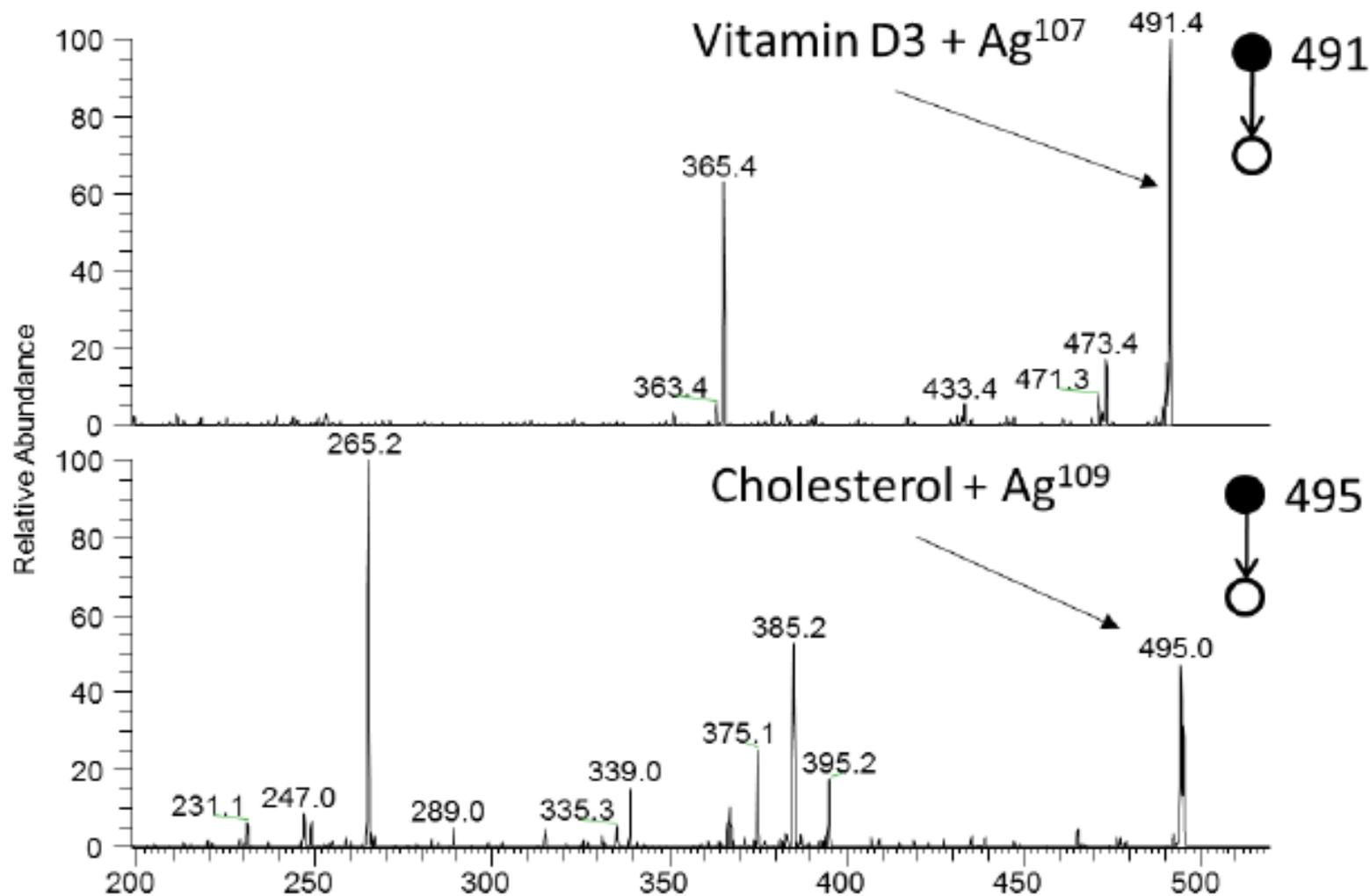
*Product ion MS/MS using CID of silver cationized cholesterol (MW=386) and vitamin D3 (MW=384). The silver cations were generated in the primary ion source using electrolytic spray under aprotic conditions.*
