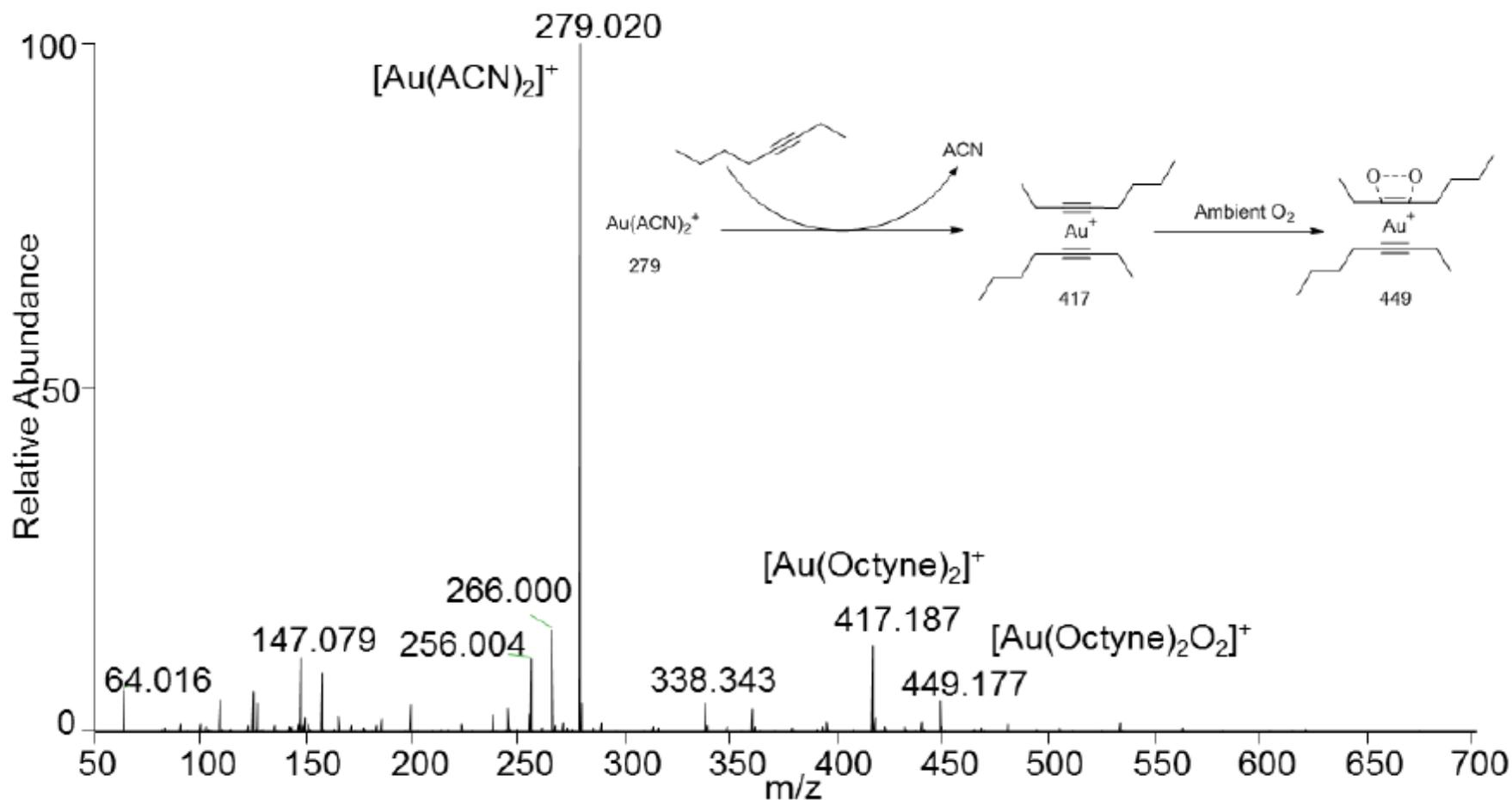
***Au<sup>+</sup> generated from electrolytic ionization of gold wire in the primary ESI source and deposited onto an alkyne (3-octyne, 100 ppbv in acetonitrile) in the secondary emitter allowed ionization by Au<sup>+</sup> clustering, ( $m/z$  417). High resolution MS confirmed the peak assignments. For the labeled peaks mass errors are all positive and smaller than 5 ppm.***
